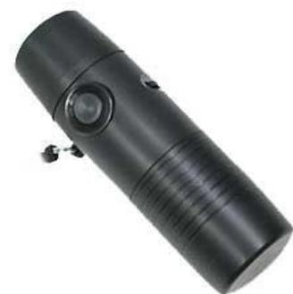
An electronic larynx (electrolarynx) is a battery operated machine that produces sound for one to create a voice. There are many different makes and types, but they are usually about the size of a small electric
